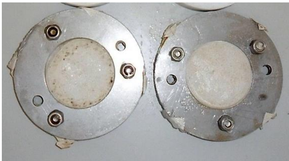
Figure 1.4 The polar organic chemical integrated sampler (POCIS) for sampling water soluble organic micropollutants from aquatic environments. Photo taken in authors laboratory in 2014.
