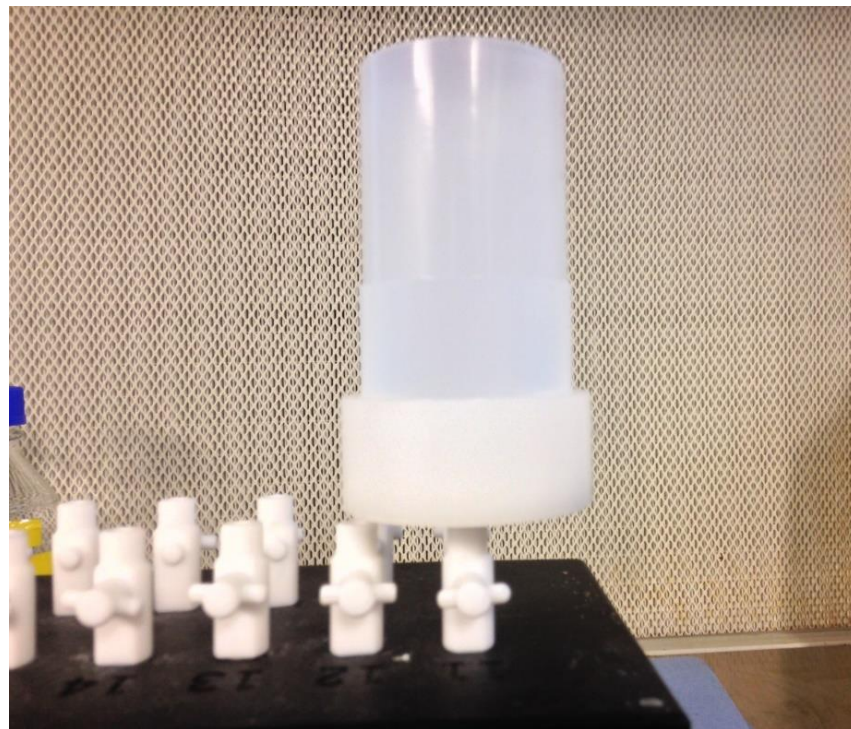
Figure 3.9 Apparatus used for the elution of adsorbed compounds from the Chemcatcher® HLB-L disk.
