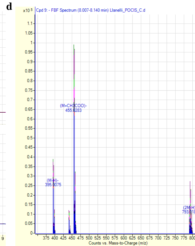
Figure 4.1 Results obtained from batch recursive feature extraction. [a] compound group table, [b] compound details table, [c(i) and c(ii)] overlaid extracted ion chromatograms for Chemcatcher® and POCIS respectively, (d) Mass spectra for POCIS.
