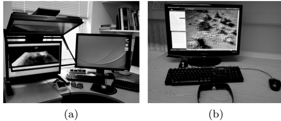
Figure 1: Example of stereoscopic visualisation: (a) a passive stereo display where images from upper and lower displays are reflected on a polarised beamsplitter in the middle; (b) an active stereo display uses a high refreshing LCD screen (120 HZ) with synchronised NVIDIA shutter glasses.
