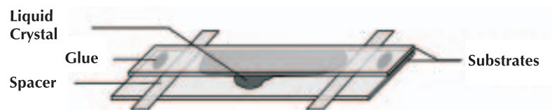
Scheme 2.2: Schematic structure of a capillary LC cell. The liquid crystal is injected in the space between the two substrates and spreads as a result of capillary forces.
