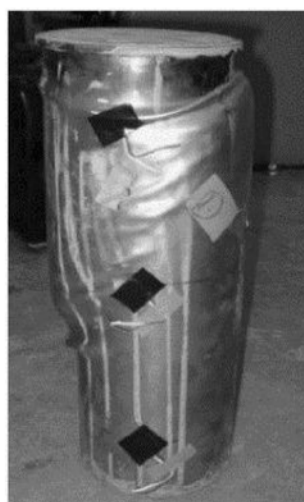
(e) Failure mode of circular CFT stub columns [16]
