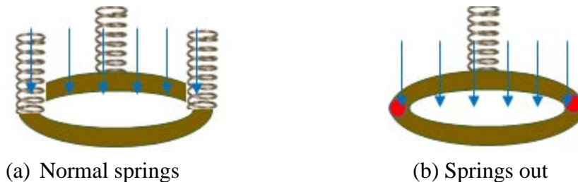
Figure 8.8 The concept of increase in the net hydraulic loaded area
