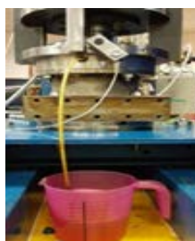
Figure 6.29 Leakage during the defective seal test
