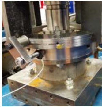
Figure 6.22 AE sensor mounted on the seal cartridge
