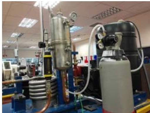
Figure 6.11 Multistage regulator mounted on the nitrogen cylinder
