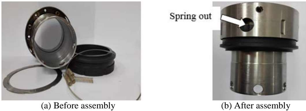
(a) Before assembly (b) After assembly Figure 6.27 Seal head assembly in spring fault simulation
