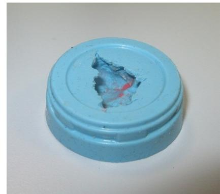
**Figure 9-24: OOMOO® ear plug cast once the plug has been demoulded**
