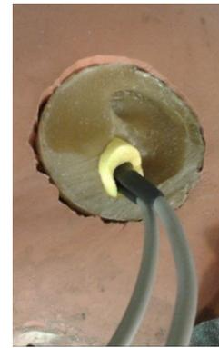
**Figure 9-17: Cheap earplug containing sensor circuit boards fitted into the modified Hybrid III dummy 'ear'**
