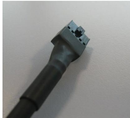
**Figure 9-36: Connector on the cable linking the ear-pieces with the data acquisition unit**
