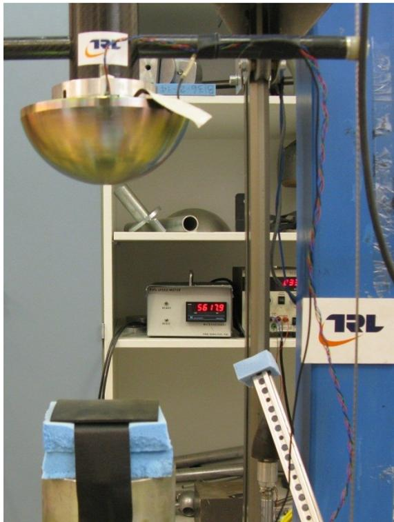
**Figure 9-4: Setup for drop tests with mini-accelerometer used in parallel with reference accelerometer.**
