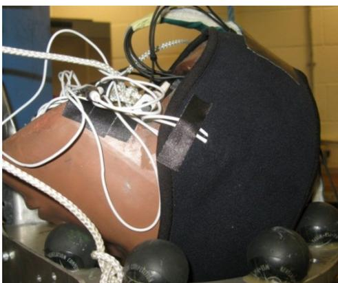
**Figure 9-29: Prototype sensor system fitted to the dummy head via a fabric headband**
