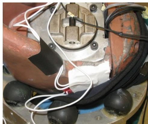
**Figure 9-30: Prototype sensor system fitted to the dummy head via a fabric plaster**
