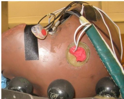
**Figure 9-28: Prototype sensor ear-piece fitted to the modified Hybrid III dummy head**
