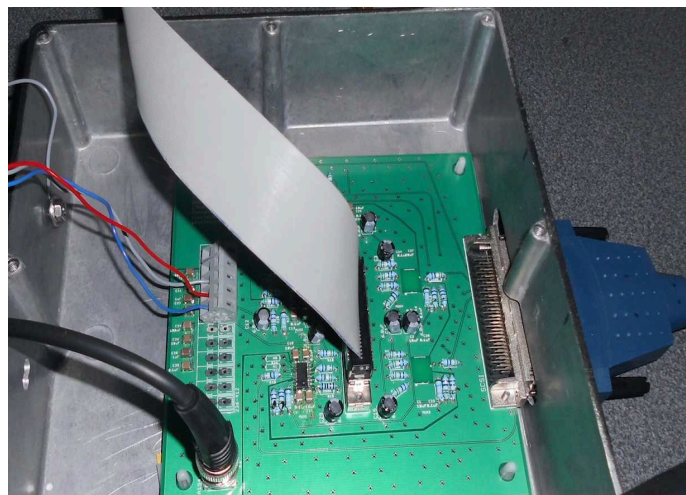
(b) Manufactured MUX PCB in a shielding box.
