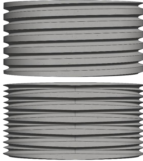
Figure 4.2. Representing homogenous grinding wheel surface after first (top geometry) and second (bottom geometry) dressing operations.
