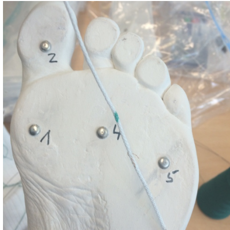
Figure 2: Temperature sensor yarn (TSY) with sensors marked in green
