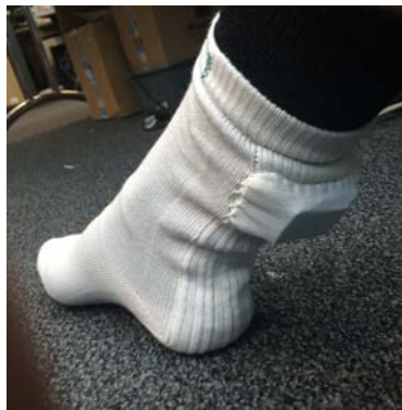
Figure 3: Temperature sensing socks developed for wear trial
