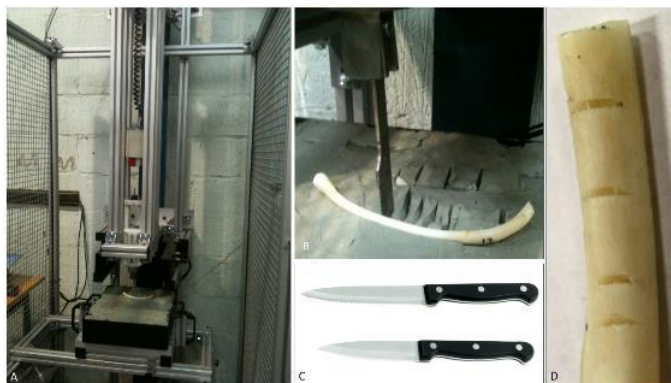
129 130 Fig. 6. A) Drop Test Rig; B) Knife marking dry rib; C) Two knives used in experiment 1, Knife 4, left and Knife 5 131 right; and D) 4 cut marks generated by Knife 4 132
