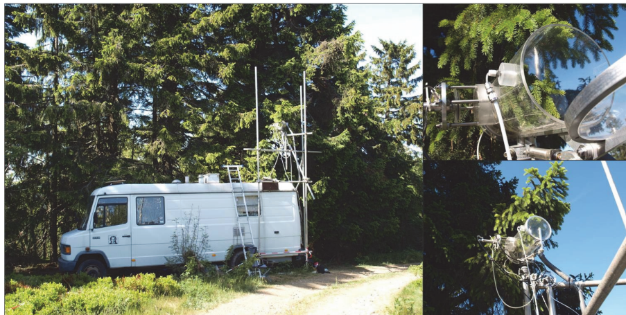
Fig. 1. Cuvette set-up in the field on Kleiner Feldberg, Taunus, Germany: The enclosure system was fixed at a Norway spruce branch. The instruments (Sensors, PTR-MS, CRM) were located in the van underneath to keep inlet lines short. For 17 min the lid was kept open to allow contact with the natural atmospheric environment and closed automatically for 3 min.
