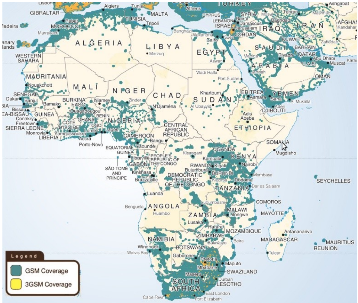
Illustration 15: GSM and 3G coverage in Africa. Latest available visualized data from end of 2007. Source: GSM Association. 2008
