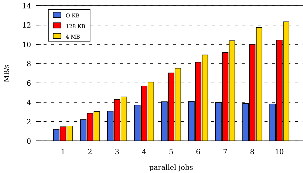
Figure 1.10 The data throughput rate at different values of the block device read-ahead. The analysis train with 15 tasks, with only AliESDs.root being accessed. Read-ahead substantially increases analysis performance for parallel jobs.
