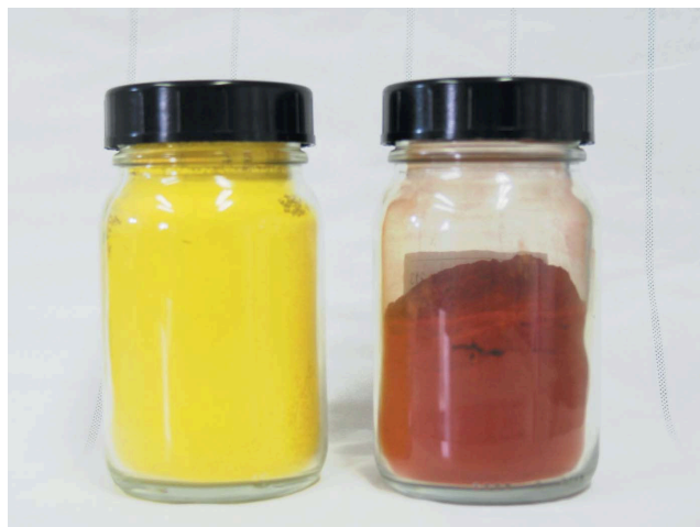
Figure 2 Pigment Yellow 213: powders of the \alpha phase (greenish-yellow) and the \beta phase (brown).
