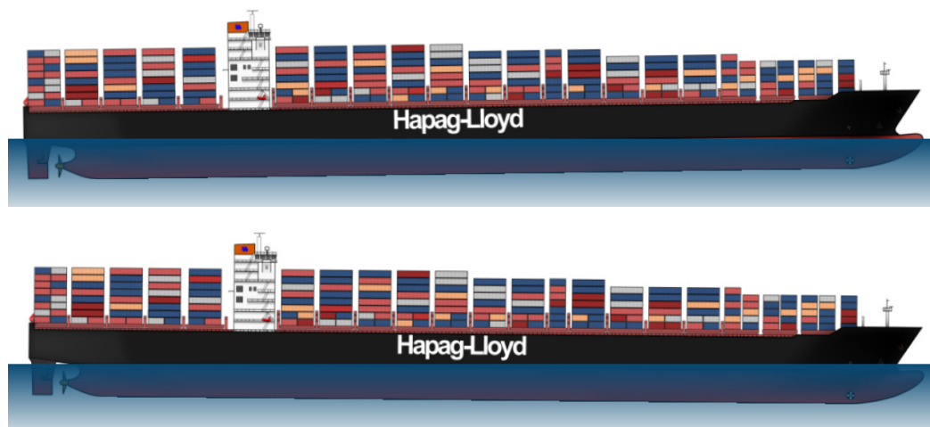
Figure 2. Visualization of different trim levels: stern trim (top) vs. bow trim (bottom). A slight bow trim will generally decrease water resistance and increase hydrodynamic efficiency (MAN Diesel & Turbo, 2011).
