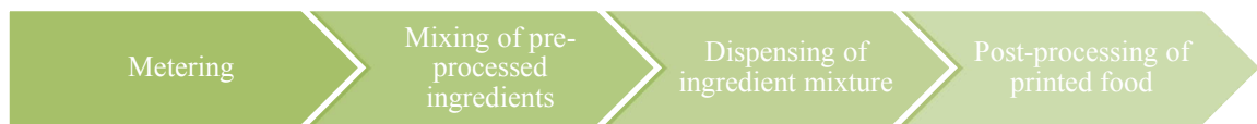
Figure 8: Four steps of AFM (Zoran and Coelho, 2011; Sun, Peng, Yan, et al. , 2015).
