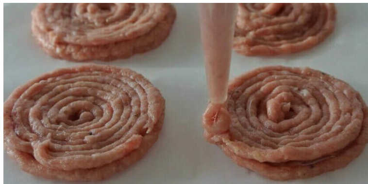
Figure 9: Soft material-extrusion 3d printing (Source: Natural Machines).
