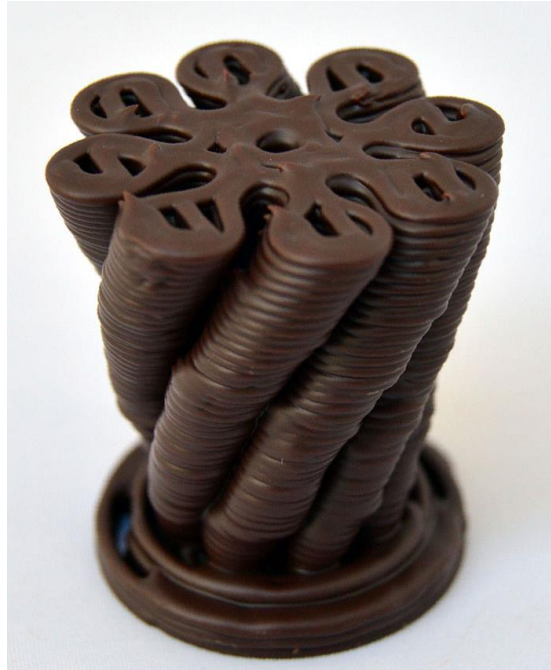
Figure 10: Chocolate structure made using melting extrusion (Source: ChocEdge).
