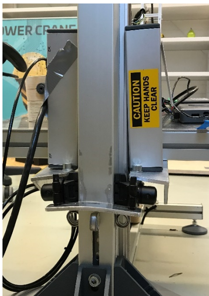
Figure 4.13 Damage to brake pad connecting plate. (replaceable part)
