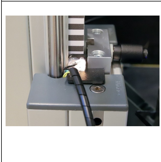
Figure 3.21 Optical encoder with white light
