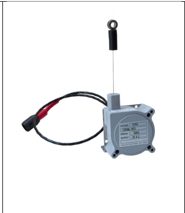
Figure 3.20: Cable-extension transducer. Due to the spring and the cable it has inertia which is not suitable for high acceleration applications. ( http://www.autometer.com/string-potentiometer-12.html )
