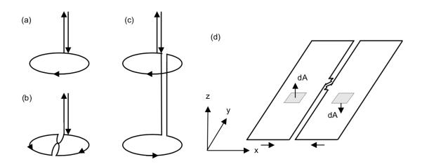
Figure 2: Flux transformer types by geometry: (a) magnetometer, (b) planar gradiometer and (c) axial gradiometer. Illustration (d) represents integration of the flux in a planar gradiometer measuring  $\Delta \mathbf{B}_z/\Delta x$  (Hansen et al. 2010, p. 32).
