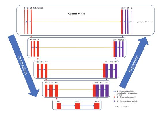
Figure 25: The custom U-Net used in approximating the MEG inverse problem.
