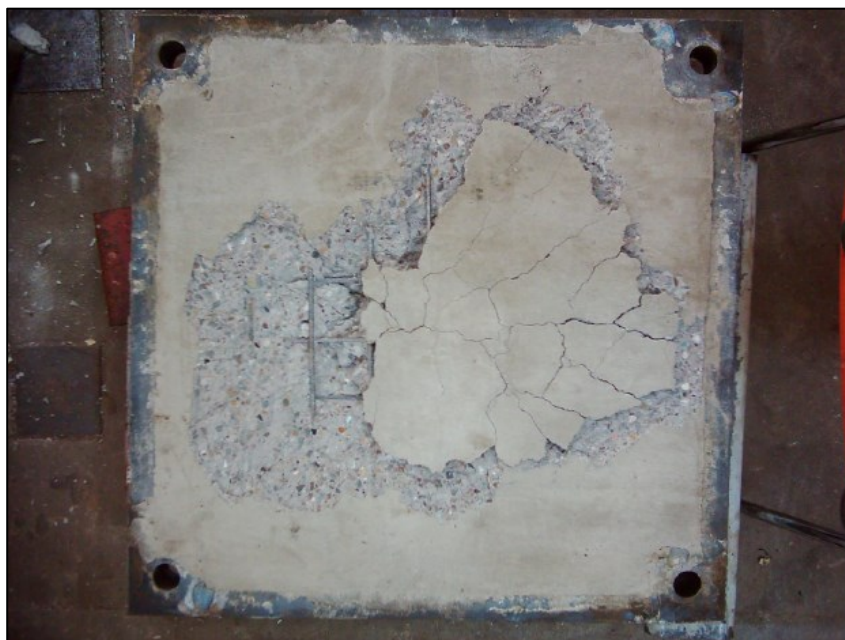
Figure 29 Distal face of the Slab S3 (No perforation) (Izatt et al., 2009)
