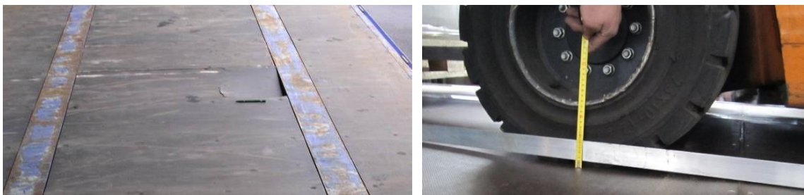
Figure 1.3: Plywood panel damaged by the forklift wheel-load (left) and semi-trailer floor stiffness measurement as per ISO 1496-1 (1990) (right). Image courtesy UPM Plywood Oy.
