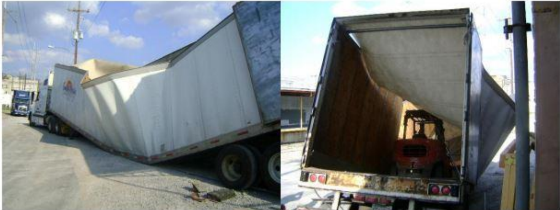
Figure 1.4: Box semi-trailer structure under forklift weight (Robson Forensic, 2017).
