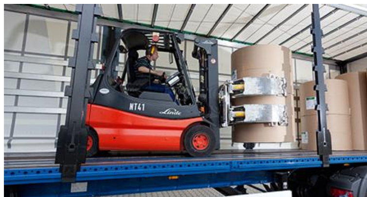
Figure 2.5: Forklift wheel-load on the semi-trailer floor (Krone, 2017).
