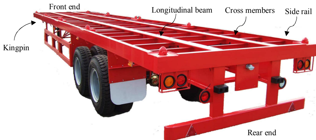
Figure 2.1: Typical flatbed semi-trailer chassis consists of two longitudinal beams connect with cross members at various locations. Image courtesy to Qingdao CIMC Special Vehicles Co. Ltd.
