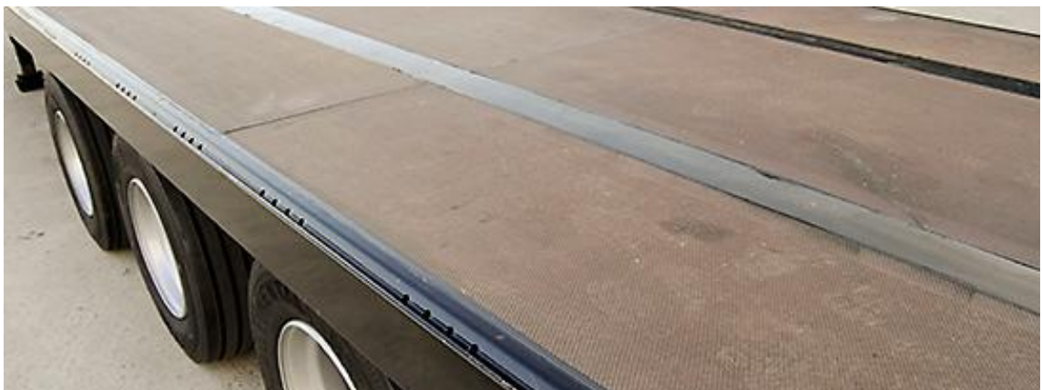
Figure 2.16: Plywood floor bonded with the semi-trailer chassis (Adhesives & Sealants Industry, 2010).
