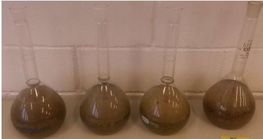
Figure 16. Sands in pycnometers during the 24h waiting time. From left to right: MS 2, NS 7, NS 1, and NS 8.
