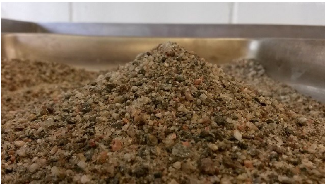
Figure 18. The achieved slope during SSD density testing for one of the sands.
