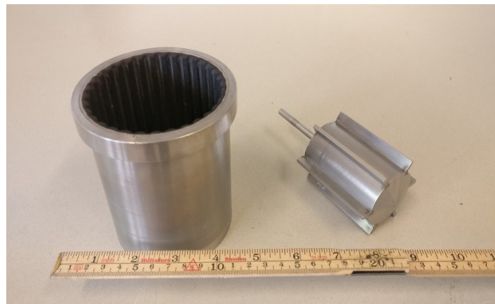
Figure 31. Cup and spindle used with viscometer.
