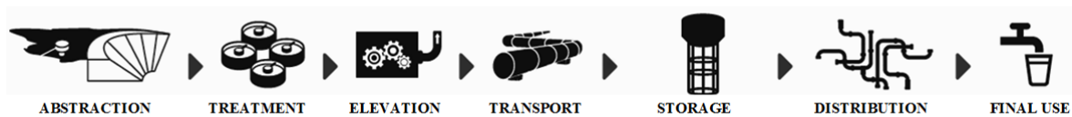
Figure 1.1: Simplified scheme of the main sections of a water supply system from the source to the end users (adapted from ERSAR, 2012).
