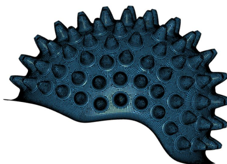
Figure 2.28: ABS cone liner proposed by Blanco et al. [2014] (adapted from Blanco et al. [2014]).
