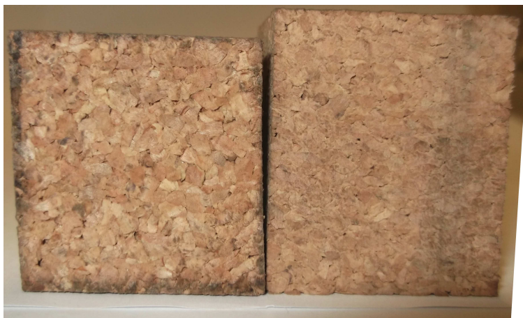
Figure 3.3: Agglomerated cork samples after and before being tested at quasi-static strain rates.
