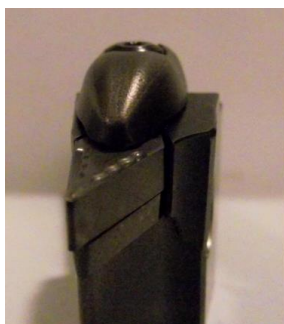
Figure 5.7 – Tool holders used in the cylindrical micro-cutting tests.
