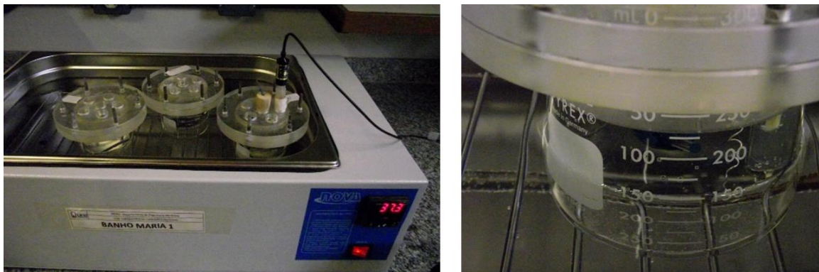
Figure 5.44 – Workpieces on thermostatic bath during the electrochemical tests.
