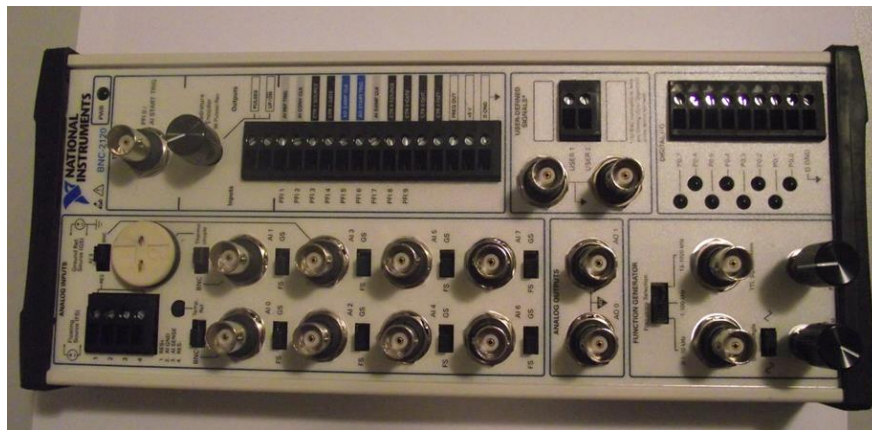
Figure 5.11 – Connector block used in the monitoring of the vibration signals.
