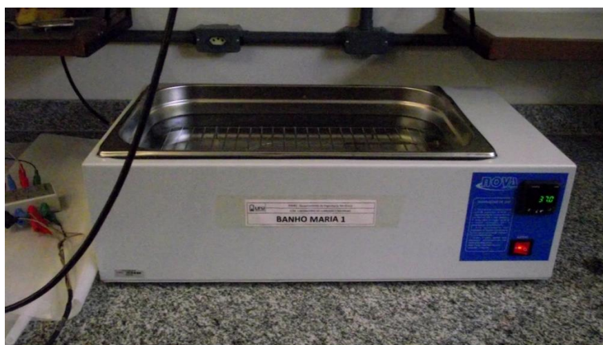
Figure 5.18 – Thermostatic bath to steady the temperature in electrochemical tests.
