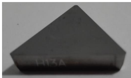
Figure 5.4 – TPGN 16 03 04 H13A inserts used in the micro-cutting tests.
