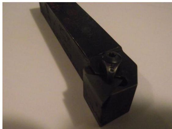
Figure 5.5 – CTGPL 2020 K16 tool holders used in the micro-cutting tests.
