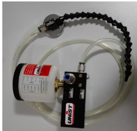
Figure 5.8 – MQL system used in the micro-cutting tests.
