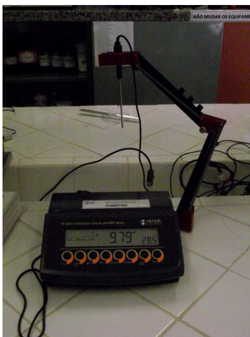
Figure 5.19 – The pH meter to measure the pH of the solution of electrochemical tests.
