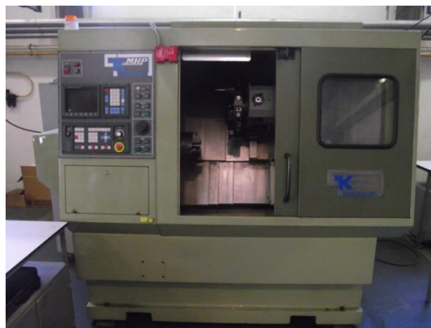
Figure 5.3 – Kingsbury™ MHP 50 CNC lathe used for the tests.
