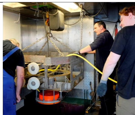
Figure 1: Installation of the 38 kHz transducer (EK80, red instrument) at the moonpool (from left to right: Peter Neumann, Olaf Willms, Florian Gausepohl). [Photo credit: Peter Urban]
