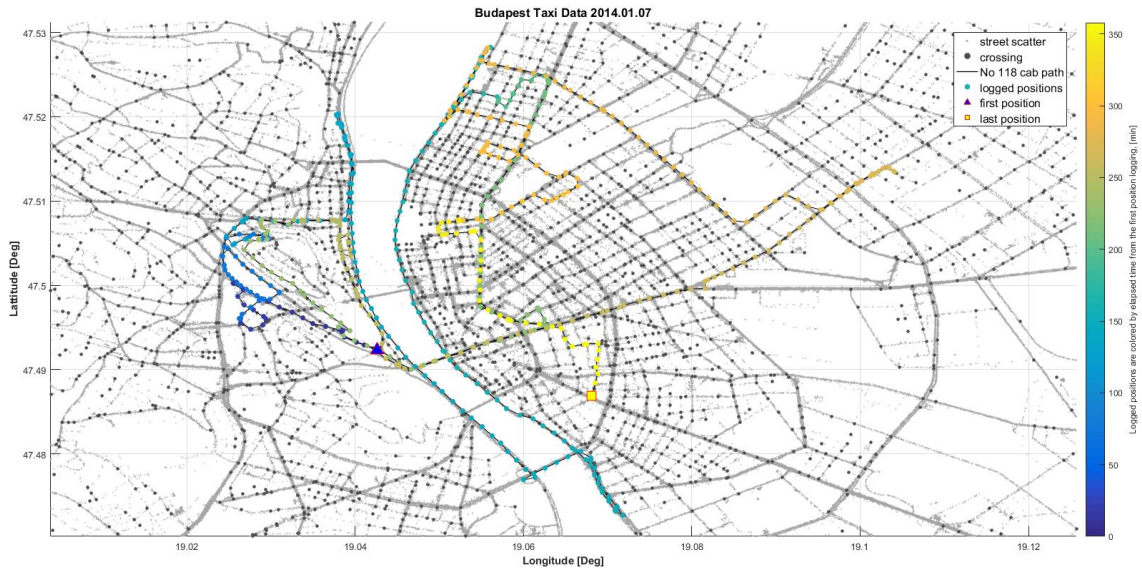
Figure 5: Scatter plot of the captured position logs ("street scatter") from all vehicles during Jan. 7., Tuesday, 2014. The position logs belonging to cab with ID No. 118. are connected and colored by the time of recording, calculated from the time stamp of the first position sample.
