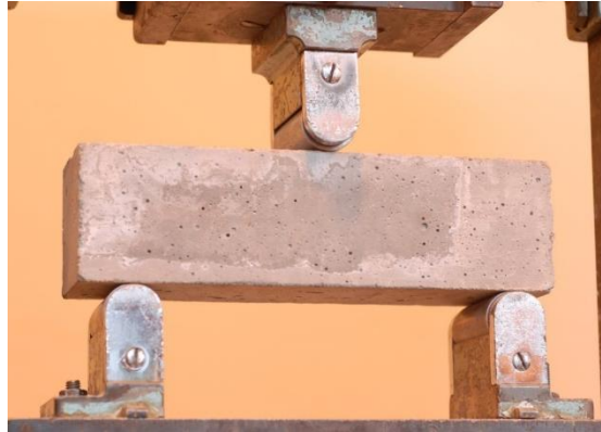
Fig. 3: Flexural strength tests (beam span=200 mm, beam length=250 mm)
