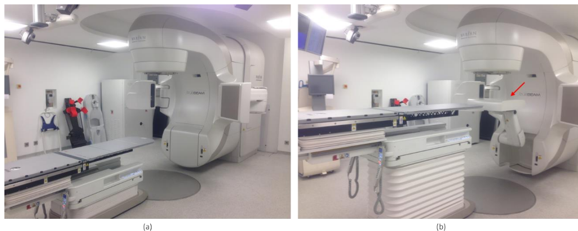
Figure 3.1. TrueBeam™ LINAC (a) without and (b) with EPID (red arrow) opened.
