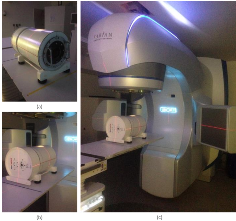
Figure 3.3. ArcCHECK viewed from (a) the front part and from (b) the back part, and (c) mounted on the LINAC. Note that in order to place ArcCHECK correctly, we have to align the lasers with ArcCHECK marks, and then with the light field.
