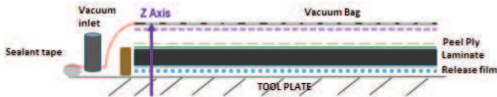
FIGURE 3. Laminating configuration and ancillary products used for manufacturing samples
