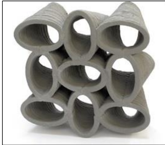
Figure 7: A complex shaped concrete section (Gosselin et al., 2016: 107)
