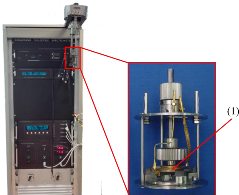
Figure III-3: Dielectric spectrometer with a temperature head mounted. The zoomed image on the right shows the location (1) where the characterization cell is placed.
