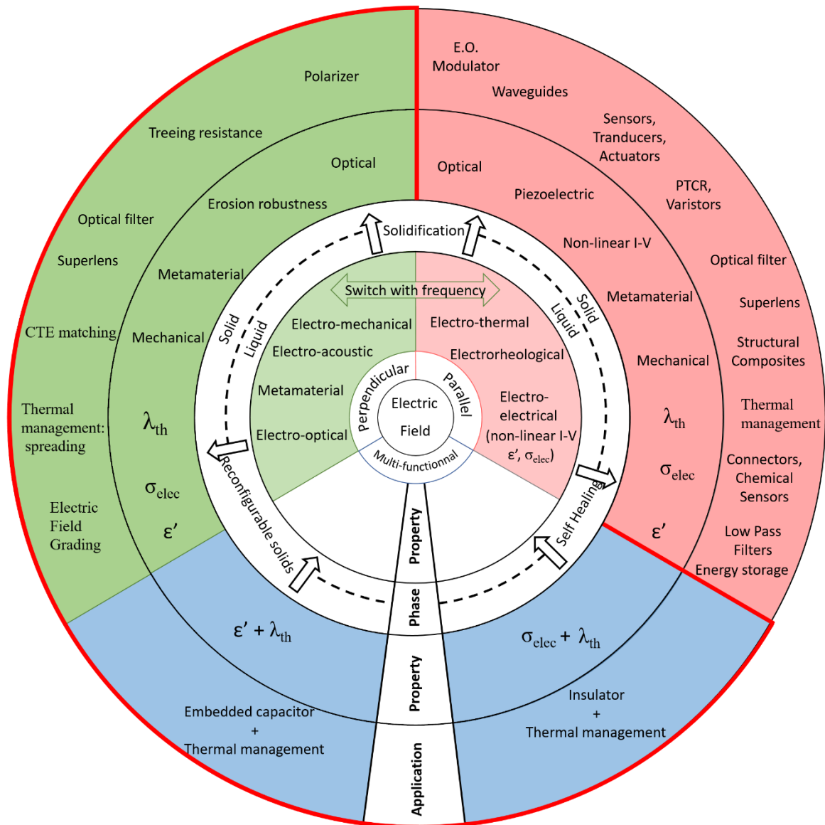
Figure VI-18: Potential applications of anisotropic, solid, and liquid composites. The inner circle corresponds to liquid composites, the outer circles to solid composites.
