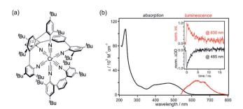
Fig. 10 (a) Chemical structure of the Cr(CN<sup>tBu</sup>Ar<sub>3</sub>NC)<sub>3</sub> complex.<sup>19</sup> (b) UV-Vis absorption and luminescence spectra of Cr(CN<sup>tBu</sup>Ar<sub>3</sub>NC)<sub>3</sub> in de-aerated THF at 20 °C. Excitation occurred at 450 nm. Inset: luminescence decay at 630 nm (red) and absorption bleach recovery at 485 nm (black) following excitation at 532 nm with pulses of ~30 ps duration. Adapted with permission from ref. 19. Copyright 2017 American Chemical Society.
