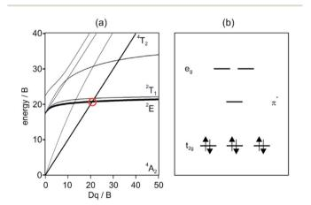
Fig. 1 (a) Tanabe–Sugano diagram for the  $d^3$  electron configuration. (b) Relevant frontier orbitals for low-spin octahedral  $d^6$  metal complexes with low-lying ligand-based  $\pi^*$  orbitals.
