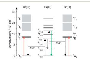
**Fig. 8** Energy-level scheme for the Cr(m)-Er(m)-Cr(m) helix from Fig. 7 illustrating the near-infrared to visible upconversion process. EnT stands for energy transfer. The dashed gray downward represents nonradiative relaxation. Reproduced with permission from ref. 30. Copyright 2012 Elsevier.
