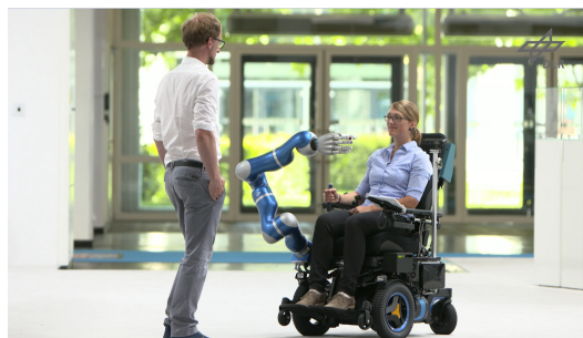
Figure 1: EMG-based Human-Robot Interaction with EDAN (demonstration with non-disabled person).
