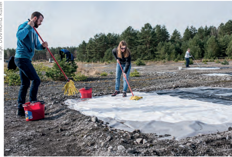
Image: DLR/Moritz Küster Tarpaulins represent the craters. They need to be spotless to help the camera correctly detect the contrast.
