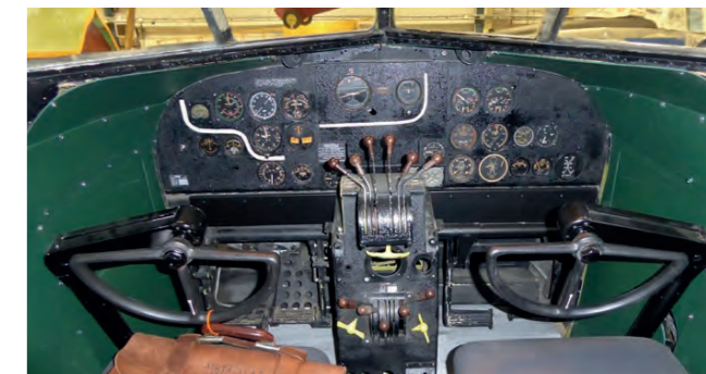
The cockpit of a small Lockheed Electra 12-26 commercial aircraft from 1942. Interesting features include the white-marked instrument area for the artificial horizon, the altimeter, the speed display, the compass and the turn-and-bank indicator.
