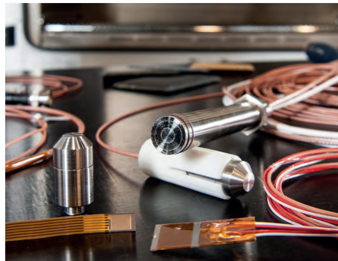
Sensors such as those in the picture ensure the quality of the component while it cures in the autoclave
