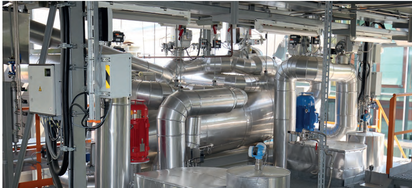
The TESIS system is designed in such a way that the flow of molten masses and their temperatures can be regulated differently depending on the test requirements
