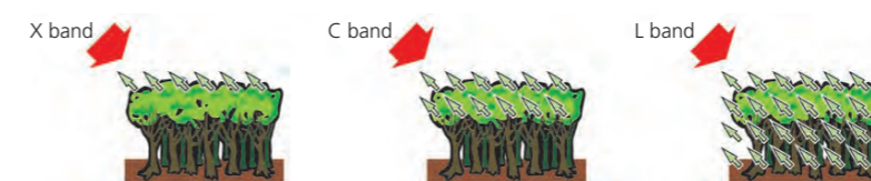
Comparison of the penetration depths in vegetation of X, C and L bands with wavelengths of three, five and 24 centimetres: While radar waves in X band are only reflected by the upper tree canopy, L band reaches the ground. Only L-band radar systems can receive signals from every part of the vegetation.
