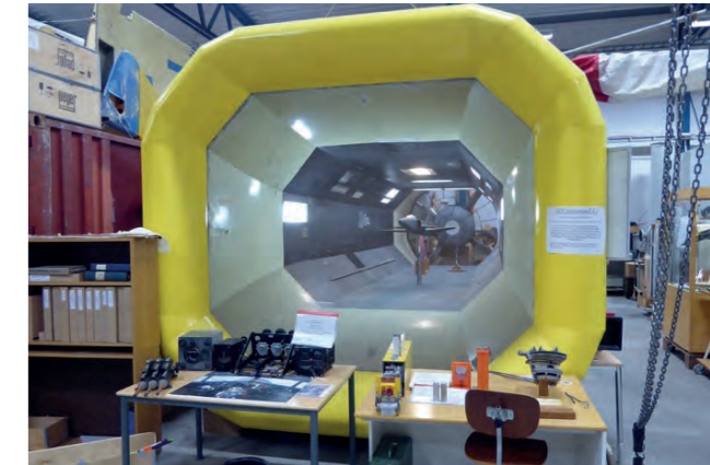
The Royal Institute of Technology's (KTH) wind tunnel carried out analyses at a wind speed of up to 40 metres per second from the 1930s onwards
