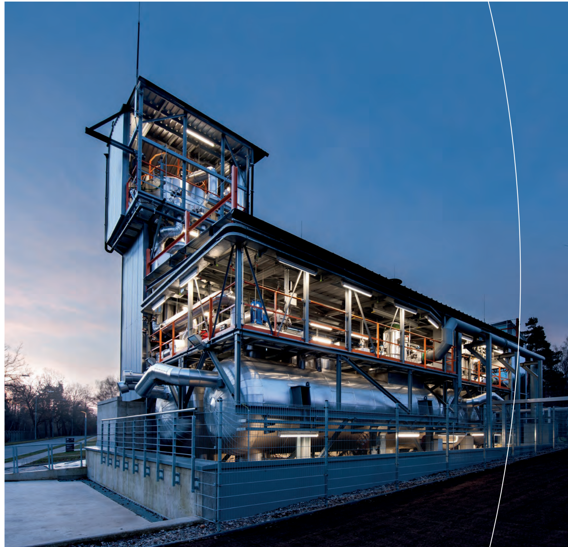
The globally unique test facility for Thermal Energy Storage In molten Salts (TESIS) enables industry to investigate components for molten salt thermal storage systems under realistic operating conditions
