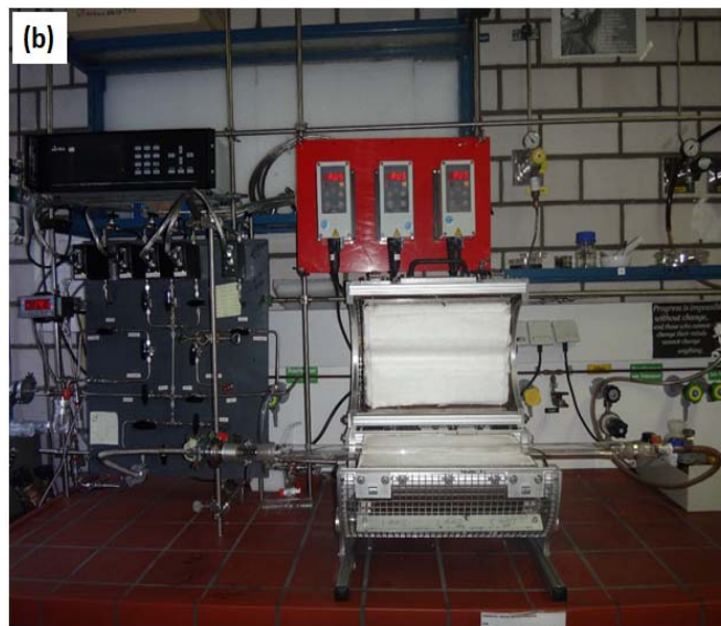
Figure VI.3 (a) Schematic and (b) photograph of the chemical vapor deposition unit.
