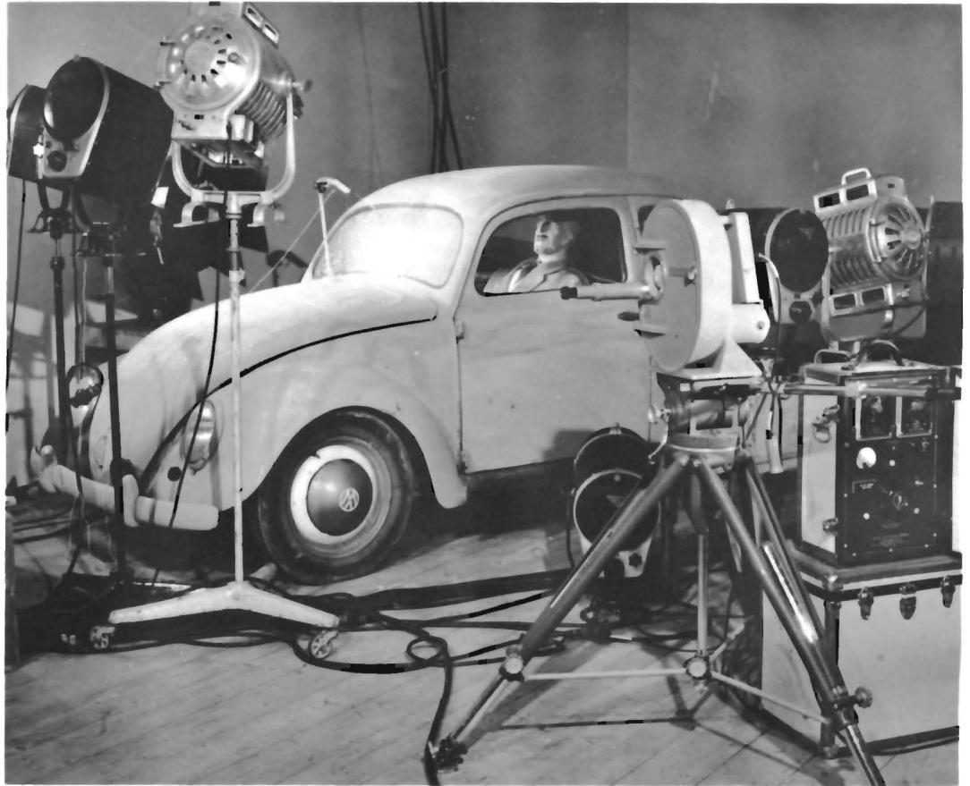
Recording of the shattering of laminated glass under impact.
