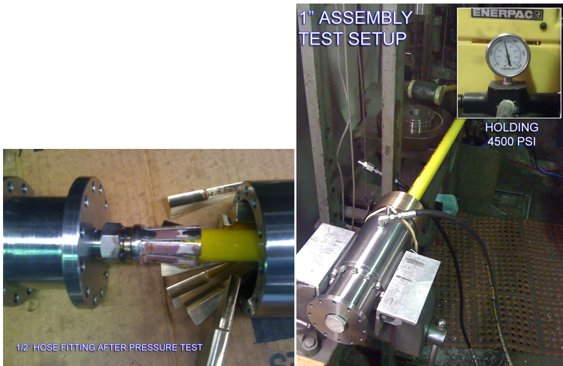
Figure 9: Production Hose Splicer unit under pressure testing
