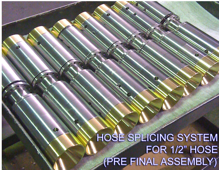
Figure 10: Assembled Hose Splicer systems readied for final assembly (handle and spring pin attach)
