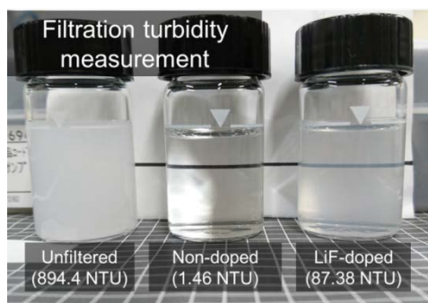
Fig. 5 Unfiltered water (894.4 NTU) and filtered water passing through non-doped (1.46 NTU) and LiF-doped (87.38 NTU) membranes.
