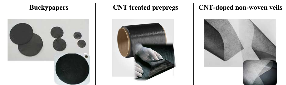
Figure 1. Three of the most promising intermediate CNT-based NEPs to be manufactured by the PLATFORM Pilot Lines (PPLs).
