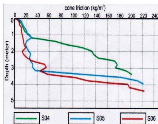
Fig 5. Cone friction (q c ) over depth at S04, S05, and S06
