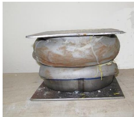
Figure 11. Combination of steel cylinder and porous filler, Type LSC-N after shortening of approximately 65% (Brunnegger, 2017)
