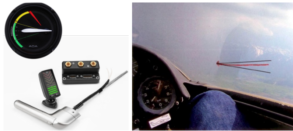
fig. 5a-b: Instruments showing angle of attack: strings used as tell-tales on gliders and sailboats.
