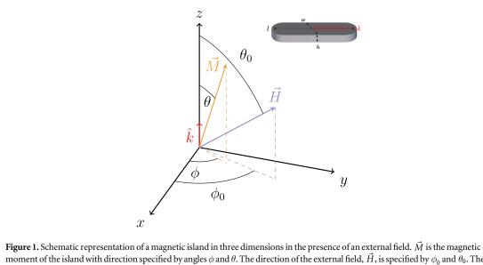
moment of the island with direction specified by angles  $\phi$  and  $\theta$ . The direction of the external field,  $\vec{H}$ , is specified by  $\phi_0$  and  $\theta_0$ . The *z*-axis is aligned with the anisotropy vector,  $\hat{\kappa}$ . The inset shows the assumed shape and dimensions of an island as well as the direction of the anisotropy axis. The dimensions of an island are taken to be h = 3.2 nm, w = 170 nm and l = 470 nm, as estimated by Farhan *et al*[10].
