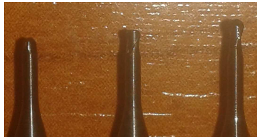
Fig.7 : Tool after wave form, after cycloid form, unworn tool
