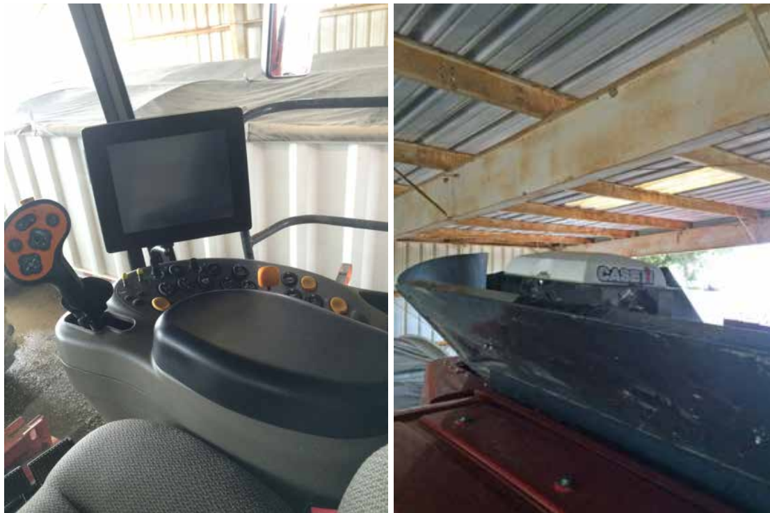
Fig. 2. AFS Pro 600 Display (left) and AFS 262 Receiver (right).
