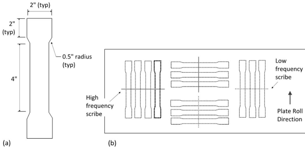
Figure 2. (a) Steel coupon geometry (b) coupon material orientations from rolled A709 plate
