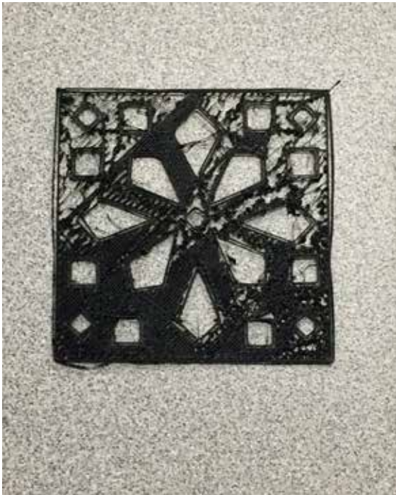
Fig. 1. Final tile designed by the authors, printed in thermoplastic polyurethane (TPU) filament.
