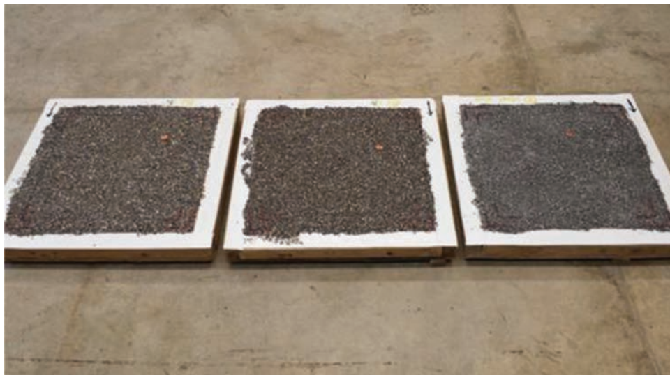
Figure 3.2 Test slabs for accelerated polishing: No. 4 calcined bauxite, No. 6 calcined bauxite, and No. 8 steel slag (left to right).
