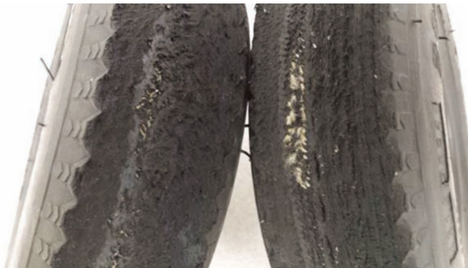
Figure 3.3 Worn out test tires by No. 8 steel slag and No. 4 calcined bauxite (left to right).
