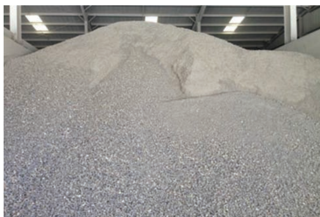
Figure 2.8 A stockpile of calcined bauxite used for HFST.
