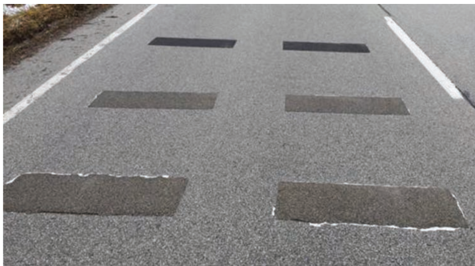
Figure 3.4 One-course No. 8 steel slag, one-course No. 6 calcined bauxite, and two-course No. 6 calcined bauxite test strips (front to back).
