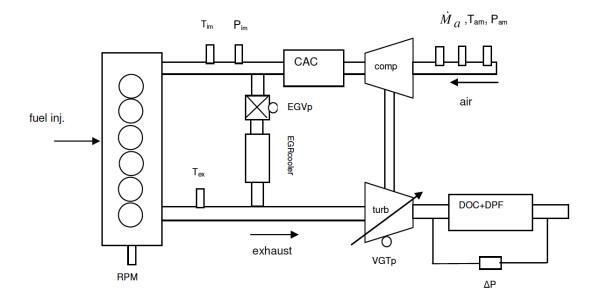
Figure 1.3. Engine architecture of reference [7] with turbocharger and EGR.
