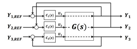
Figure 1.1. Example of decentralized control structure.
