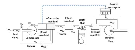
Figure 1.6. Schematic of the Caterpillar G3500 engine architecture.
