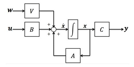
Figure 4.1. Block diagram representation of Caterpillar's state-space model.
