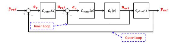
Figure 2.2. Example of nested controller with inner and outer control loops.
