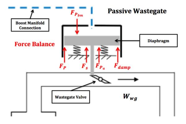
Figure 3.1. Wastegate schematic zoom-in.
