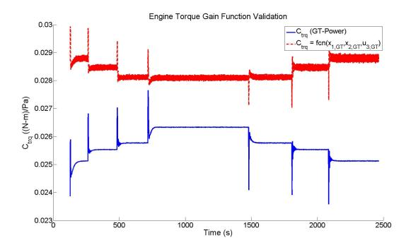
Figure 2.4. Engine torque gain expression validation.
