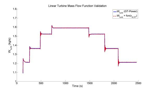
Figure 2.8. Linear turbine mass flow expression validation.
