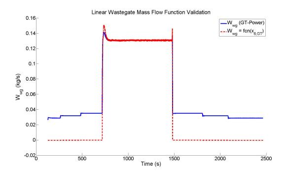
Figure 2.11. Linear wastegate mass flow expression validation.
