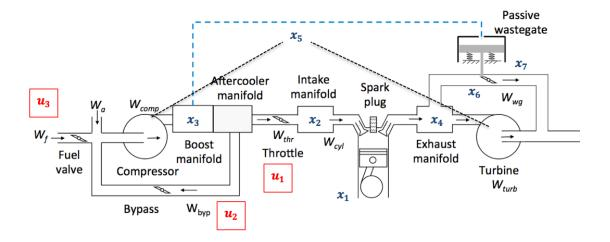
Figure 2.1. G3500 engine schematic with state and input variables.
