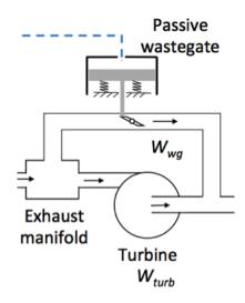
Figure 2.9. Passive wastegate schematic.
