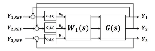
Figure 1.2. Example of decoupled control structure with pre-compensator  $W_1$ .
