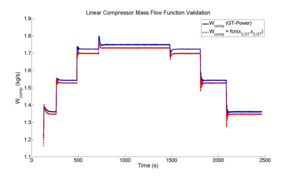
Figure 2.6. Linear compressor mass flow expression validation.
