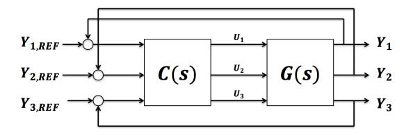
Figure 1.5. Example of centralized control structure.
