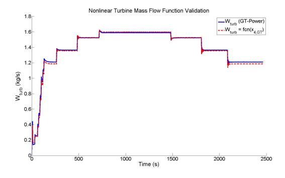
Figure 2.7. Nonlinear turbine mass flow expression validation.
