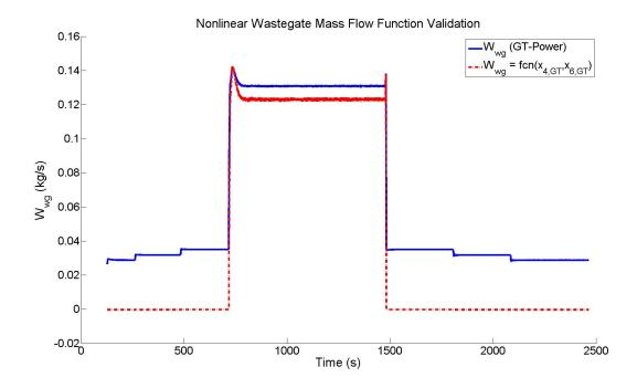
Figure 2.10. Nonlinear wastegate mass flow expression validation.
