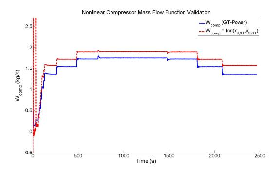
Figure 2.5. Nonlinear compressor mass flow expression validation.
