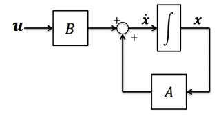
Figure 3.2. Block diagram representation of linearized physics-based engine model.
