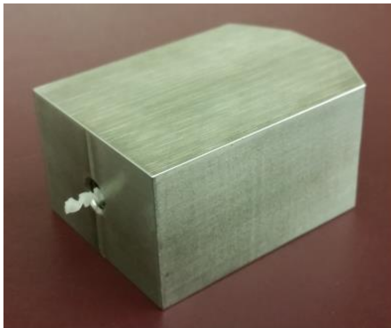
Figure 12. Protruding end of the static mixer before the needle has been screwed into place.
